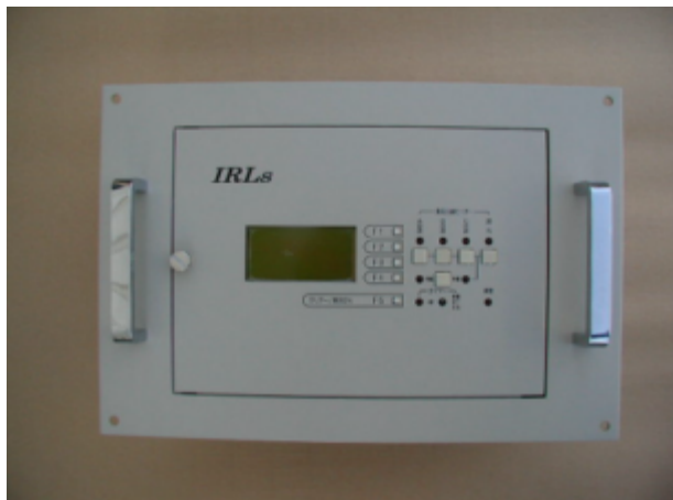
IRL s (Intelligent Road Lighting System)
