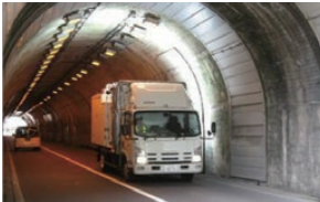
Wall surface image measurement using mobile image measurement vehicle
