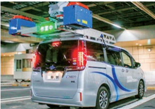
Vehicle with automatic survey of pavement conditions
