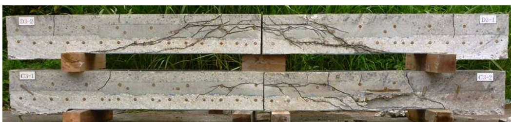
(c) NT8+C (42.6 万回で破壊)
